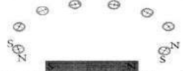
Drawing a magnetic field line with the help of a compass needle
