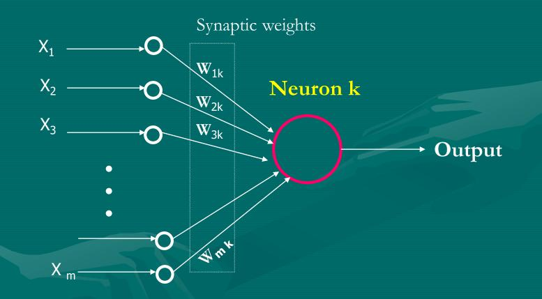
**Learning** occurs by changing the effectiveness of synopsis which are modeled as weights iii. Weighted sum of inputs (WSI) : is called the net input to a Neuron The net input to neuron' k is given by  $\mathbf{v}_k = \sum_{j=1}^m \mathbf{w}_{kj} \mathbf{x}_j$
