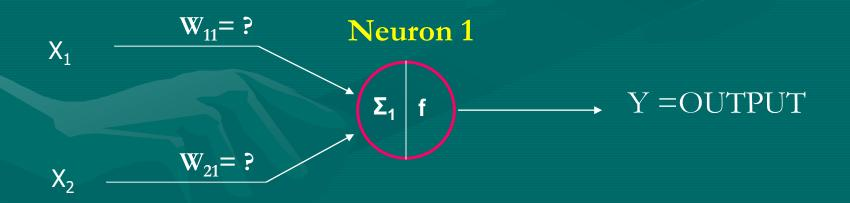
Note: The objective in the design of NN is adjusting the weights
