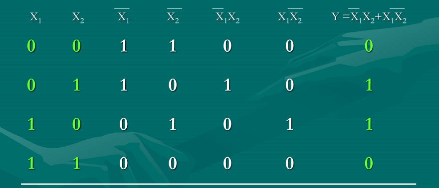
Note: The above construction is to know the Input and Output
