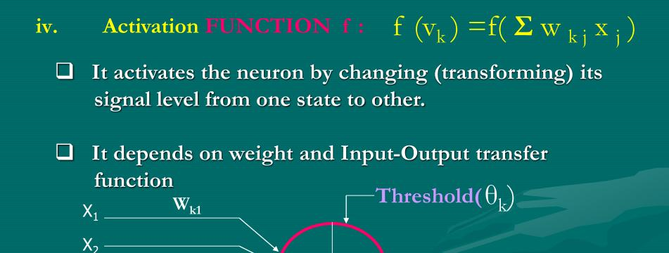
This function falls typically into one of three categories: Linear, Threshold and Sigmoid
