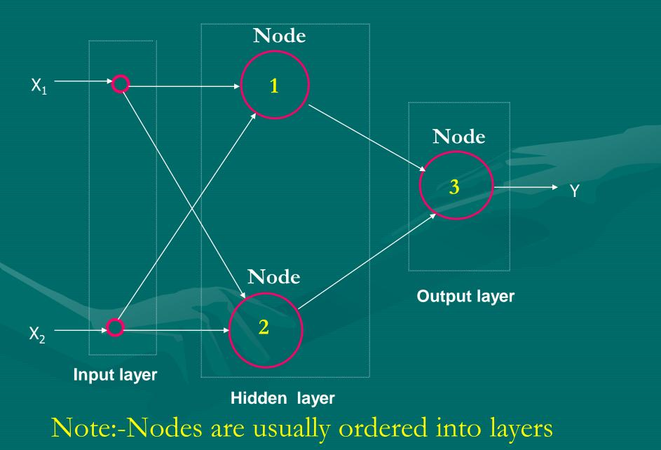
Step III:- ADJUST WEIGHTS and Fix Threshold Assign values to Weights (Hit and Trial Method being followed) Let W11= -1, W12 =1, W21=-1, W22=-1 W13= -1, W23= -1 Linear Combiner : Weighted Sum of Inputs WSI for Node 1=X1.W11+X2.W21 WSI for Node 2=X1.W12+X2.W22 WSI for Node 3=01.W12+02.W23 Apply Threshold Activation FUNCTION Threshold for Node 1=-0.5, Node 2=1.5 and for Node3 = -0.5
