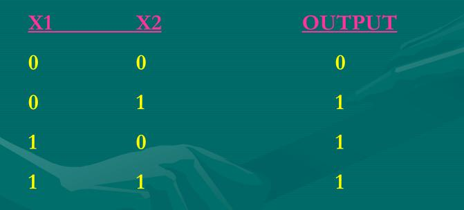
Note: Given input and output ,find f i.e determine the "system"
