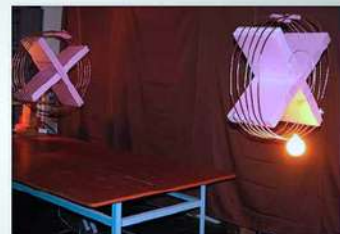
Experiment demonstrated at MIT. A 60W light bulb lit from source at a distance of 2m from load.
