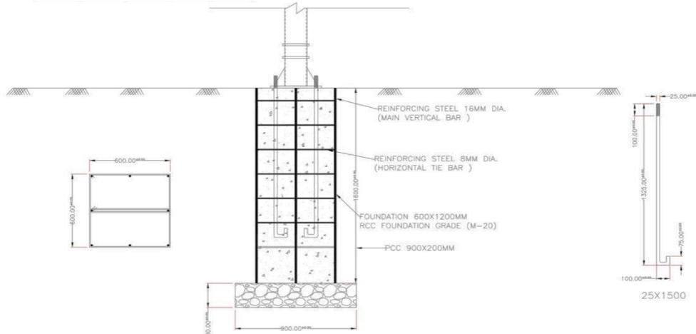
Note:-All dimensions are critical & in mm. Please maintain the dimensions. Welding dimension should be maintained 5 mm.
