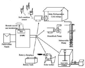
The solar pumping system with USPC can be used for agrarian applications such as water pumping, apple grading and polishing system, wheat (grain) flour grinding machine/aata chakki, cutter/chaff, deep-fridge/cold storage, blower fan for cleaning of grains, heating loads and any other standard voltage (400/415V) three phase motor/equipment of capacity not more than the capacity of Solar PV pumping system. Further, the applications are not limited upto the few shown in the figure.
