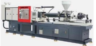
shall provide the facility to manufacture the lid/covers of variable size to these units. Units will be required to provide raw material and mould of their requirement at CFC to get their job work done. A 250 injection moulding machine has been proposed.
