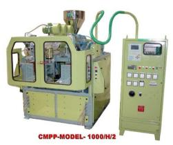
With this technology, the CFC will be able to provide facility to cluster units to manufacture HDPE/PVC bottles. Cluster units shall be required to provide their raw material required and user fee to get their work done. The bottles will be further processed (labelling, capping etc.) at individual unit level.
