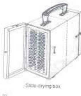
Box used in the field to dry blood smears
