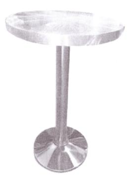
Material = 304 grade stainless steel Table top diameter = 24 inches Height of table top from ground = 42 inches To be supported by at least one stainless steel post of 3 inches diameter Base of post(s) to be firmly bolted onto / embedded into the concrete floor. Table top shall be made of 14 gauge stainless steel. Thickness of moulded edge of table top shall be 2 inches.
