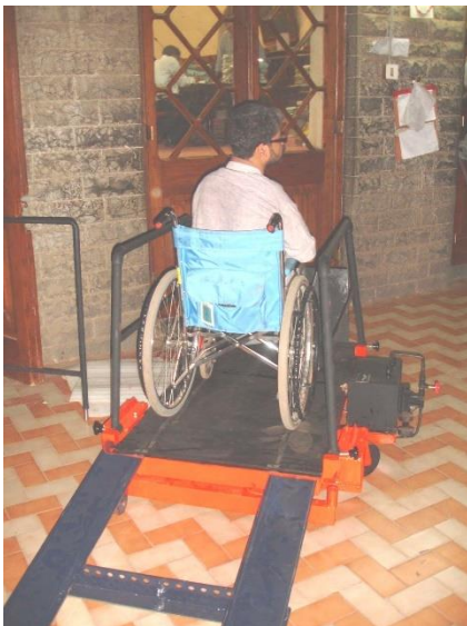
Portable Hydraulic Ramp installed in Bombay High Court
