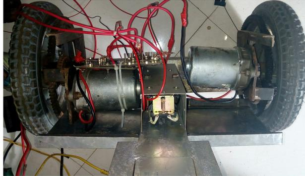
Figure 7.1: DC motor intergated with 12 inch wheels for Mobility Vehicle
