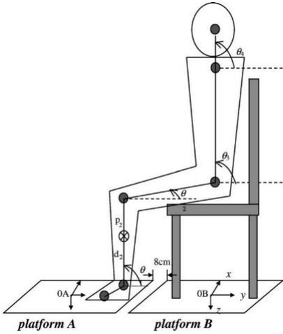
Figure 1.3: Schematic description of the four-joint, five-segments presentation of the human body, including the feet, lower legs (shanks), upper legs (thighs), trunk and head[2]
