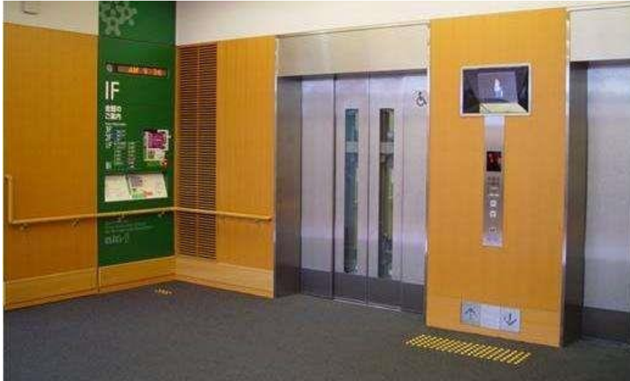
Photo 10-1. Lift signage and colour contrasted amenities
