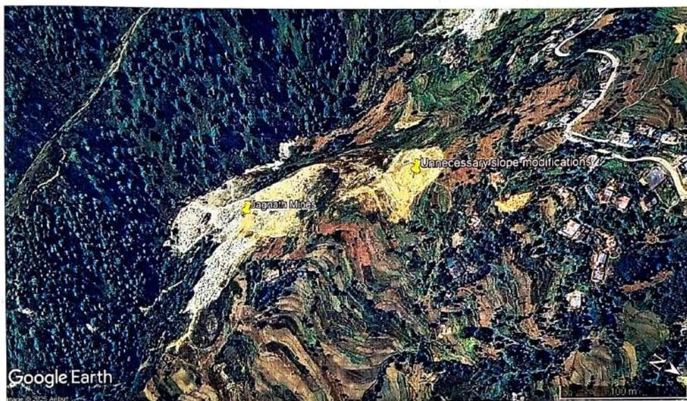
Fig. 3: Unwarranted slope modification in the unmineralized rock.
