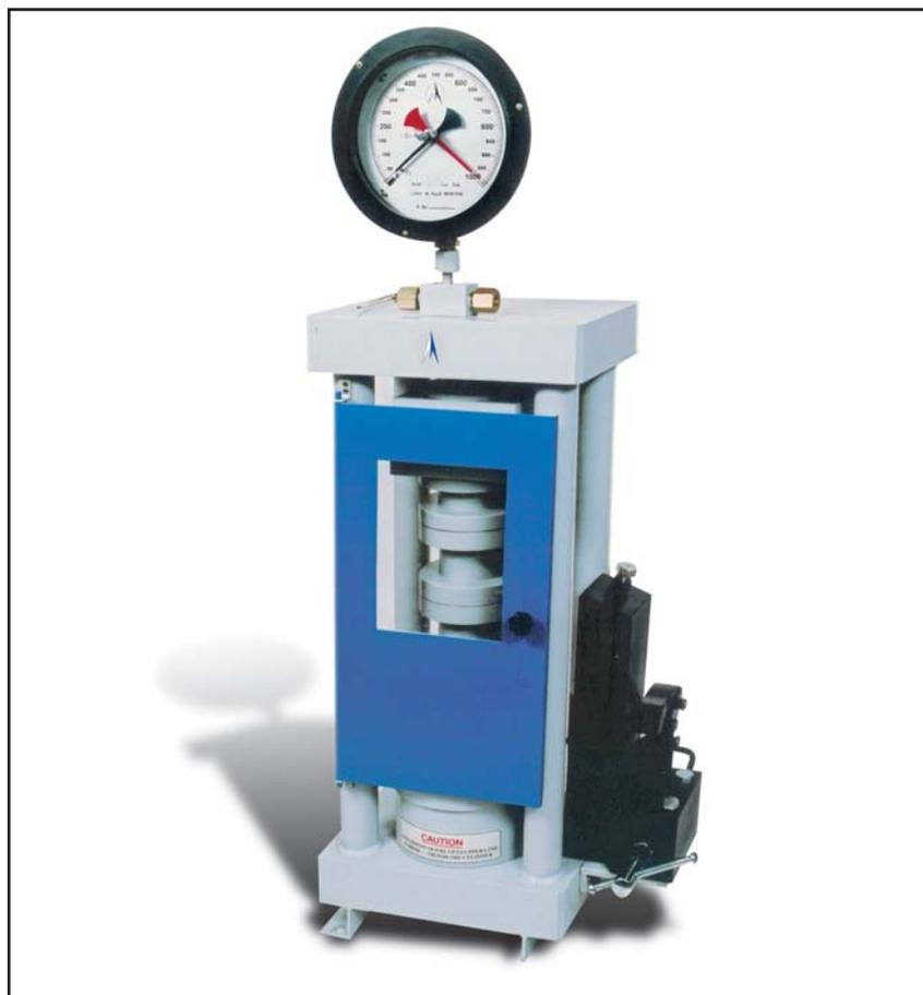
**HAND OPERATED COMPRESSION TESTING MACHINE**
