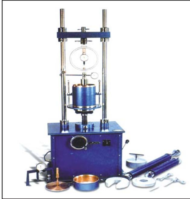
LABORATORY CBR TEST APPARATUS
