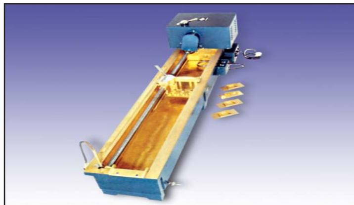
**Ductility Test Apparatus**
