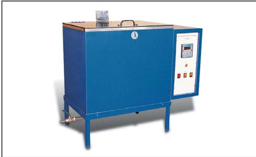
ACCELERATED CURING TANK
