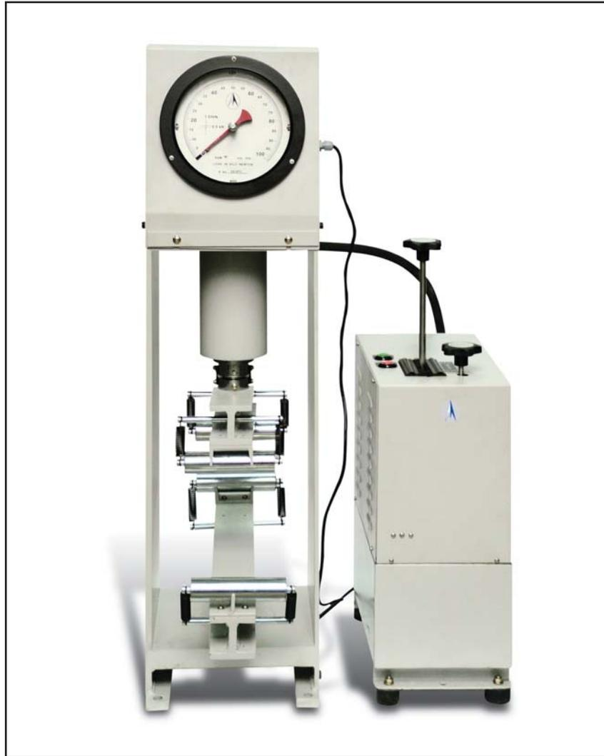
**FLEXURE TEST APPARATUS**
