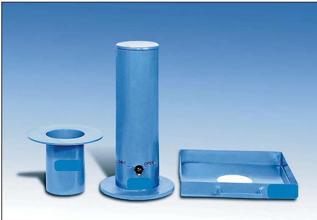
**SAND POURING CYLINDER APPARATUS**
