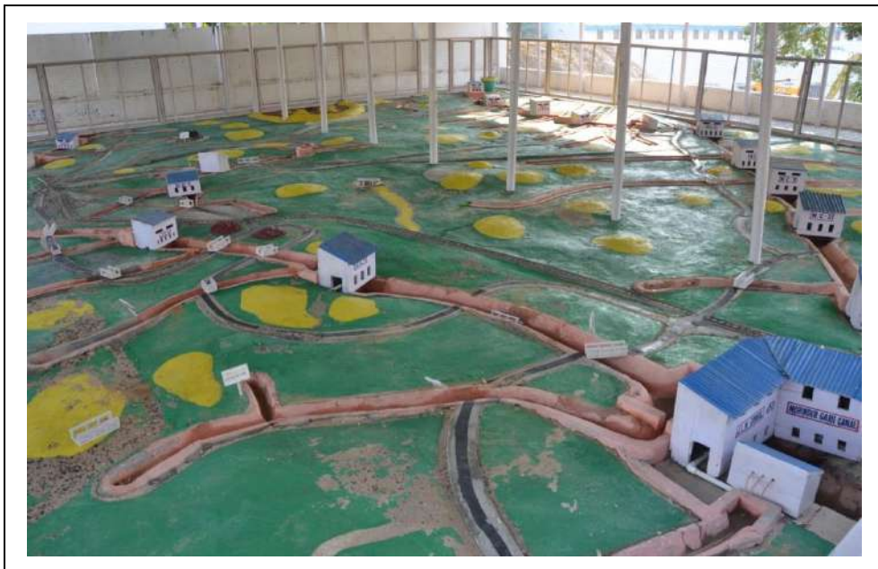
Working model installed to explain the cumulative lift of 464.04 feet under lift irrigation project and showing the related canal network of Jhajjar Water Services Circle at JF2, Salhawas
