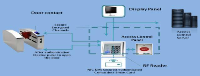
A Proof of Concept was successfully carried out at NIC premises for Access Control System using SCOSTA-CL cards as requested by MHA. ECIL and NIC jointly carried out the PoC. On successful authentication with the user's SCOSTA-CL card, the Photograph along with demographic detail was displayed on the monitor, and the flap barrier gate was opened.
