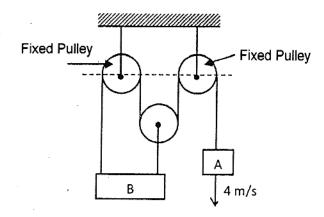
Two blocks A and B are connected by a string via pulleys as shown in the figure. If the block A moves downward with a velocity of 4 m/s, what will be the velocity of block B?
