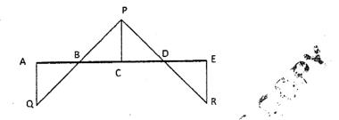
The bending moment diagram of a simply supported beam, supported at both ends is shown in the figure. In that case, which of the following figures shows the nature of shear force distribution in the beam? It is given that AB = BC = CD = DE and |AQ| = |PC| = |ER|.
