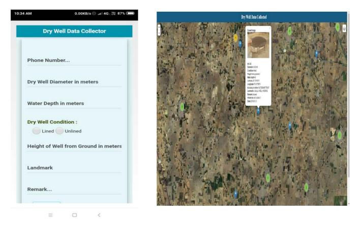
Fig.3. A view of Android based Mobile App used for mapping of dry wells
