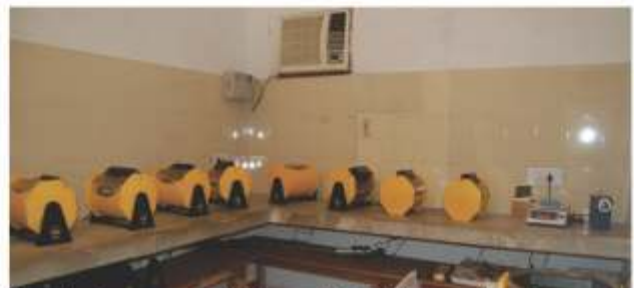
Incubator room with forced air table-top incubators.
