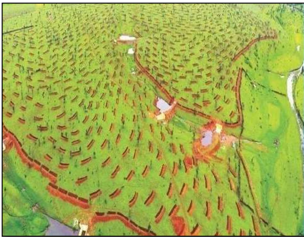
Fig 3.6: Staggered Trenches (SGT)
