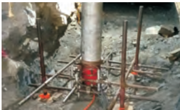
LVDT's setup for Uniaxial Jacking Tests
