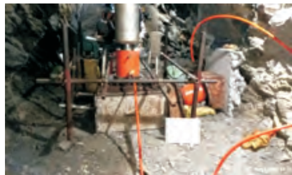
Setup of In-situ Shear Test
