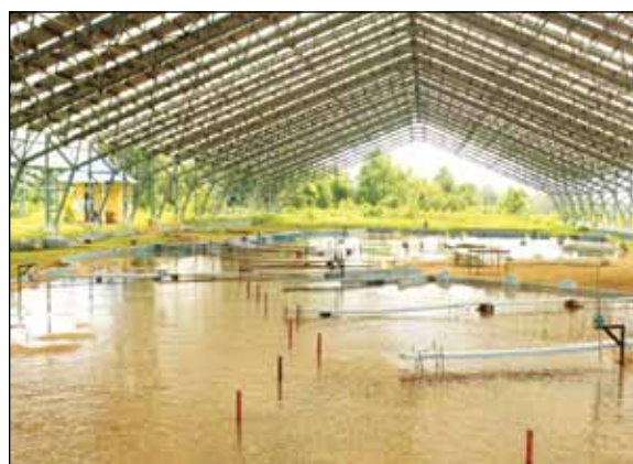
North Eastern Hydraulic and Allied Research Institute (NEHARI)- Study of Physical Model in the covered Model Tray- Brahmaputra Board
