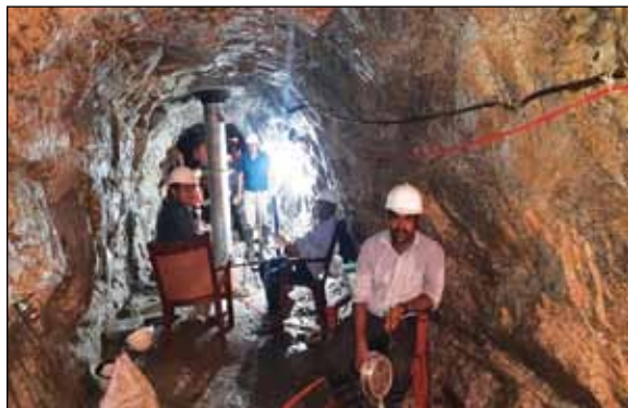
Uniaxial Jacking Deformation Test
