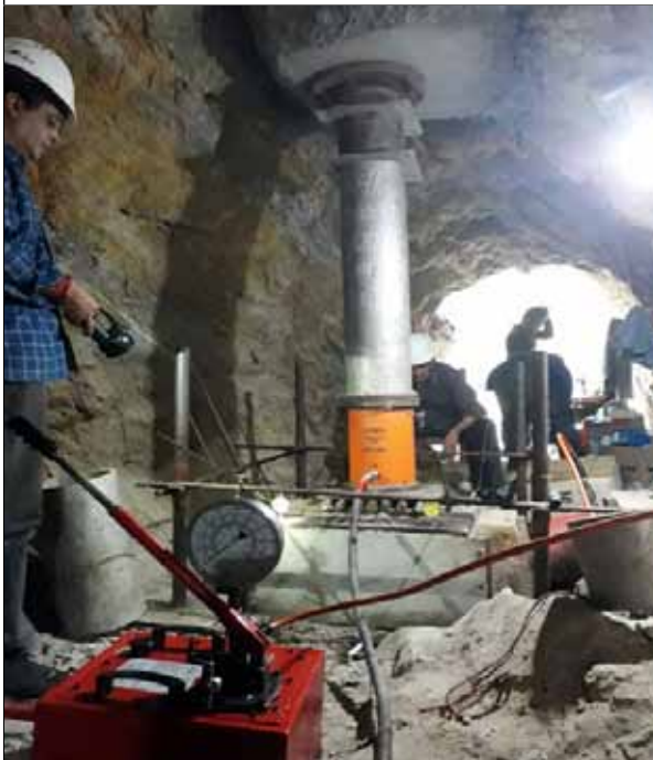
In-situ shear test in progress
