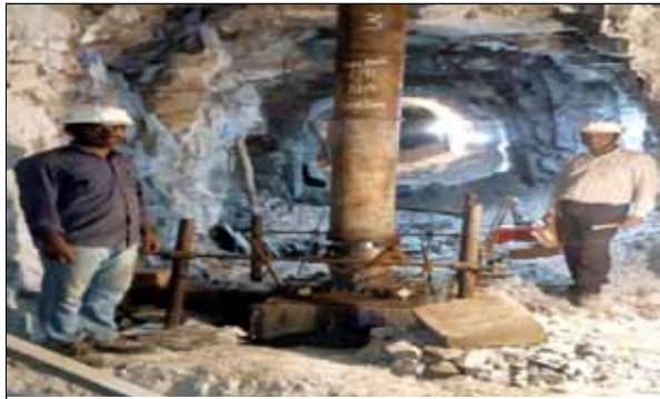
In-situ shear test in dam site drift
