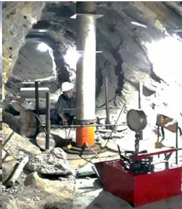
In-situ plate load test in progress
