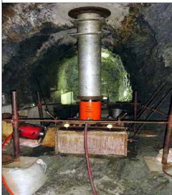
In-situ shear test in progress
