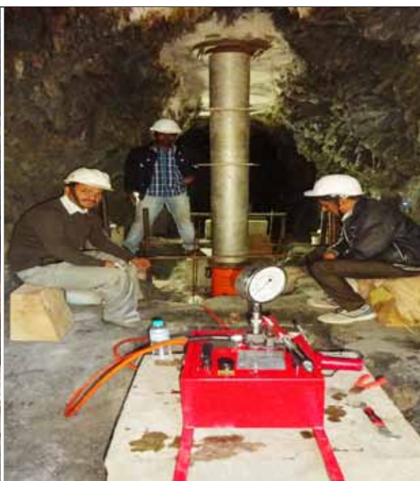
In-situ plate load test in progress
