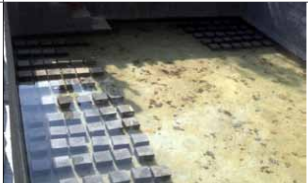
Concrete cubes in curing tank
