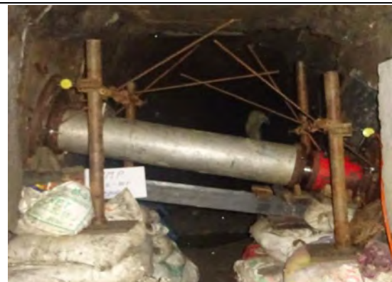
Uniaxial Jacking Test at Pancheshwar Multipurpose Project, Nepal/ India
