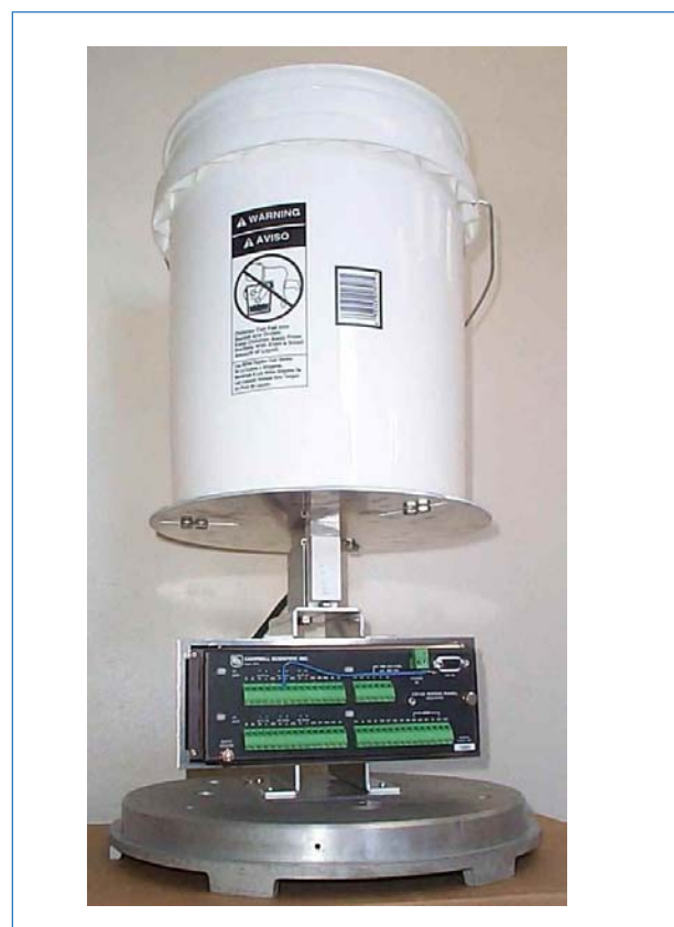
FIGURE 2.3: A) A FROZEN PRECIPITATION GAUGE WITH UP TO 1,500 MM CAPACITY (LEFT); B) WITH 1,000 MM CAPACITY (ABOVE)
