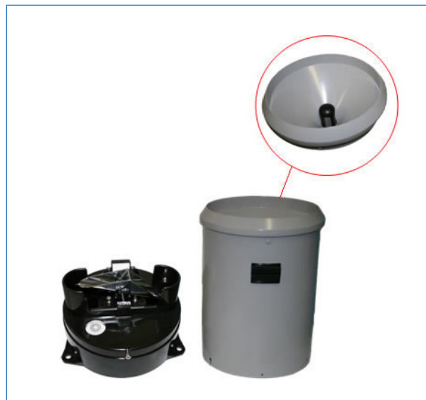
FIGURE 2.2: A TIPPING BUCKET TYPE RAIN GAUGE WITH A SIPHON SYSTEM
