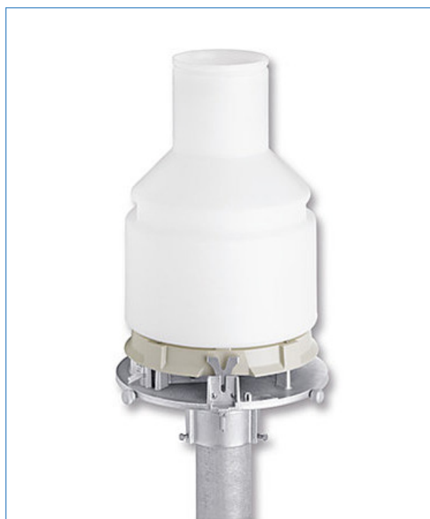
FIGURE 2.3: A) A FROZEN PRECIPITATION GAUGE WITH UP TO 1,500 MM CAPACITY (LEFT); B) WITH 1,000 MM CAPACITY (ABOVE)
