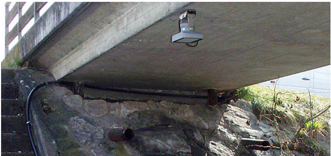
FIGURE 3.6: AN ULTRASONIC SENSOR BEING USED TO MEASURE WATER ELEVATION USING A BRIDGE MOUNT
