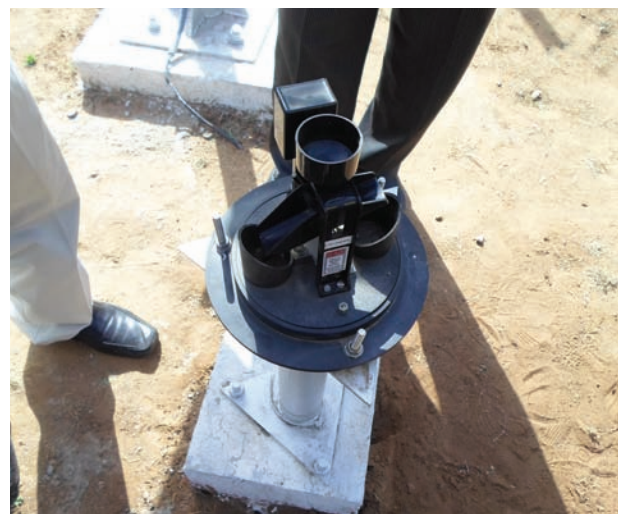
FIGURE 2.1: A) A TYPICAL TIPPING BUCKET RAIN GAUGE (TOP); B) A 0.5 MM BUCKET INSTALLED DURING HYDROLOGY PROJECT (HP)-II (ABOVE)
