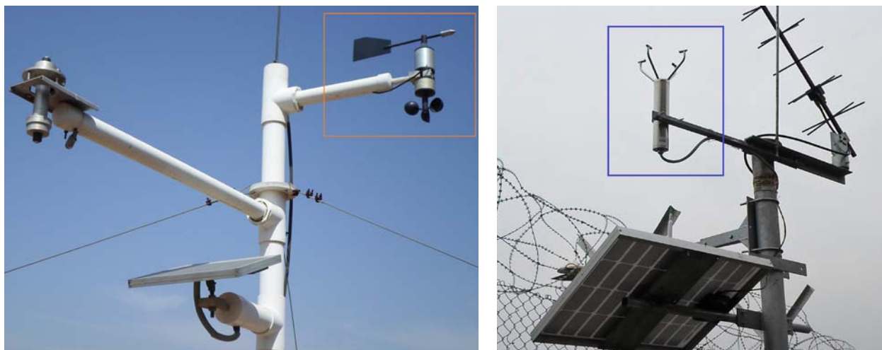
FIGURE 2.9: AN ULTRASONIC WIND VELOCITY AND DIRECTION SENSOR (LEFT) AND A CUP-ANEMOMETER AND WIND VANE-BASED WIND VELOCITY AND DIRECTION SENSOR (RIGHT)
