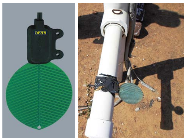
FIGURE 2.12: A) A LEAF WETNESS SENSOR (LEFT); B) A WEATHER STATION EQUIPPED WITH LEAF WETNESS SENSOR IN GUJARAT (RIGHT)
