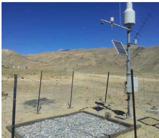
FIGURE 2.6: B) A SNOW MEASUREMENT STATION. PRECIPITATION, TEMPERATURE, SNOW DEPTH, AND SNOW PACK WATER EQUIVALENT SENSORS INSTALLED IN CHUMAR DURING HP-II
