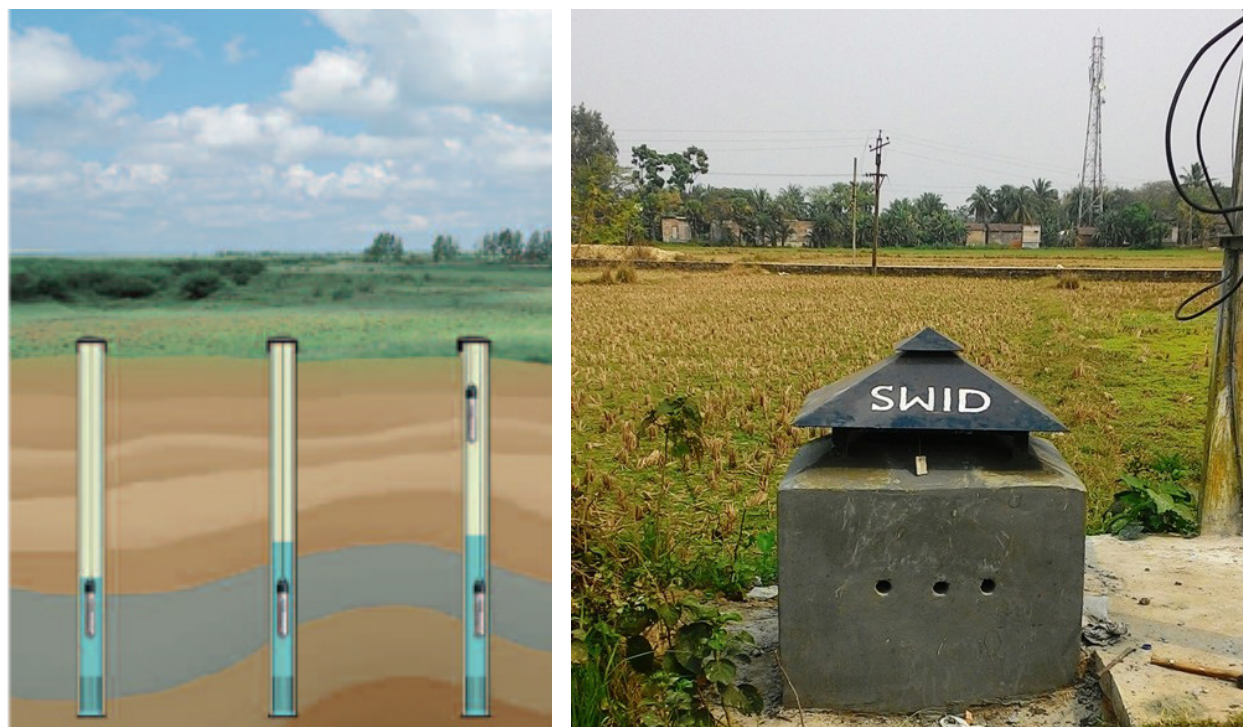
FIGURE 4.1: A) WATER LEVEL RECORDERS INSTALLED IN MULTIPLE AQUIFERS (LEFT); B) THE SECURED STRUCTURE FOR TELEMTRY DESIGNED BY THE STATE WATER INVESTIGATION DIRECTORATE, GOVERNMENT OF WEST BENGAL (RIGHT)
