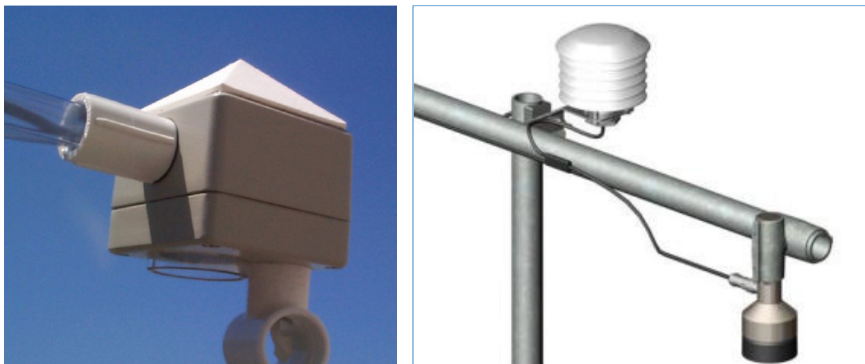
FIGURE 2.5: A) A SNOW DEPTH SENSOR SHOWING THE TEMPERATURE COMPENSATION DEVICE (LEFT); B) AN INSTALLATION WITH AN INDEPENDENT TEMPERATURE SENSOR (RIGHT)
