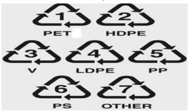
NOTE: PET-Polyethylene terephthalate, HDPE-High density polyethylene, V-Vinyl (PVC), LDPE- Low density polyethylene, PP-Polypropylene, PS-Polystyrene and Other means all other resins and multi-materials like ABS (Acrylonitrile butadiene styrene), PPO (Polyphenylene oxide), PC (Polycarbonate), PBT (Polybutylene terephalate) etc.
