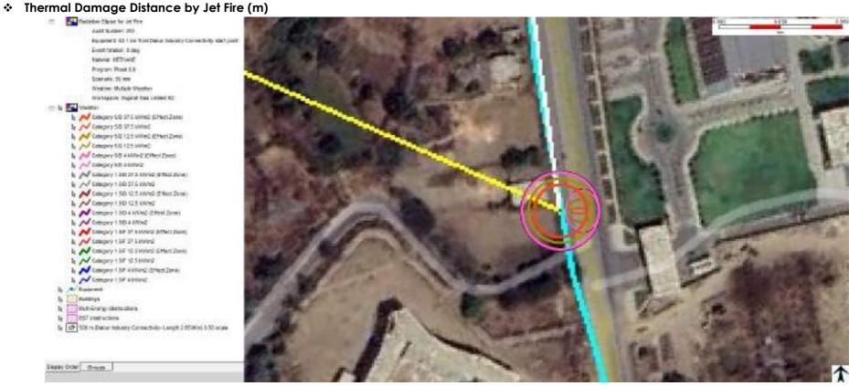
Figure 7.16 50 mm leak & 1.5D weather condition
