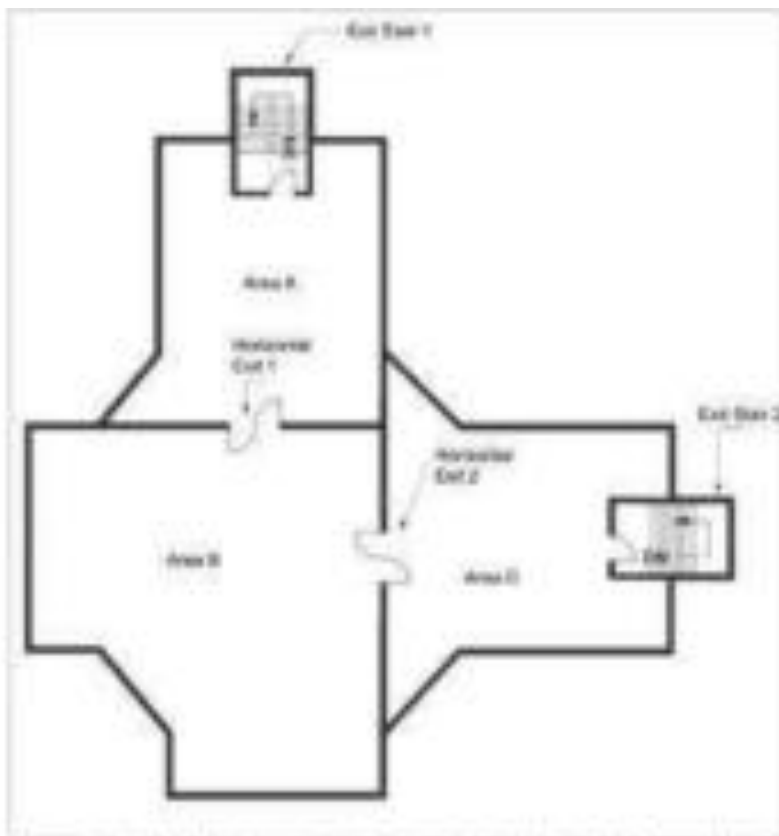
Figure No. 14.10. Minimum of Two Exits Accessible from all Parts of Floor
