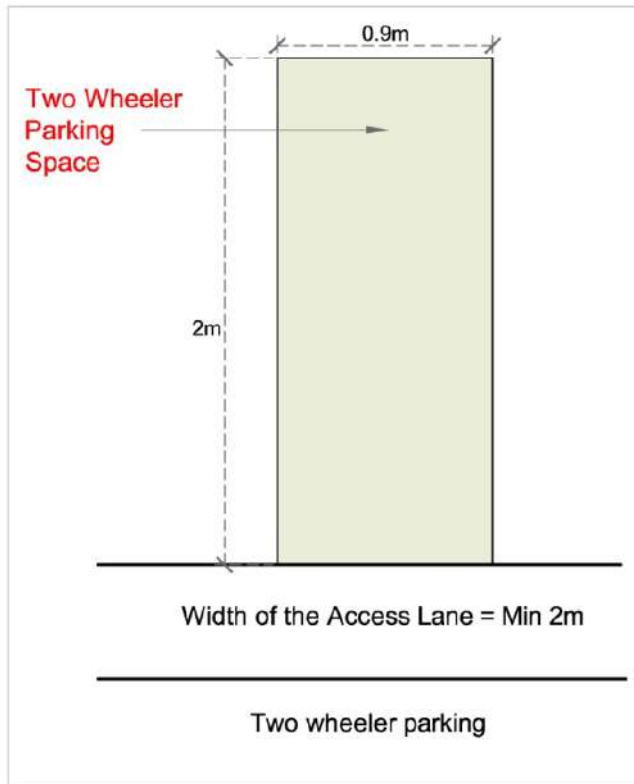
Figure No. 13.19: Design of Parking for Two - Wheelers
