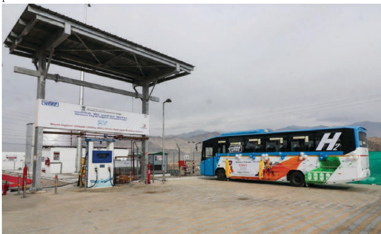
Figure 7.11 (b) Hydrogen Fuelling Station (altitude- 3650m MSL) & Hydrogen Fuel Cell Bus
