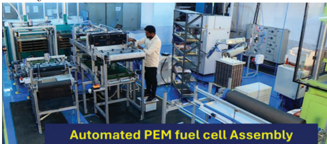
Figure 7.12 Automated PEM fuel cell Assembly at ARCI-CFCT, Chennai
