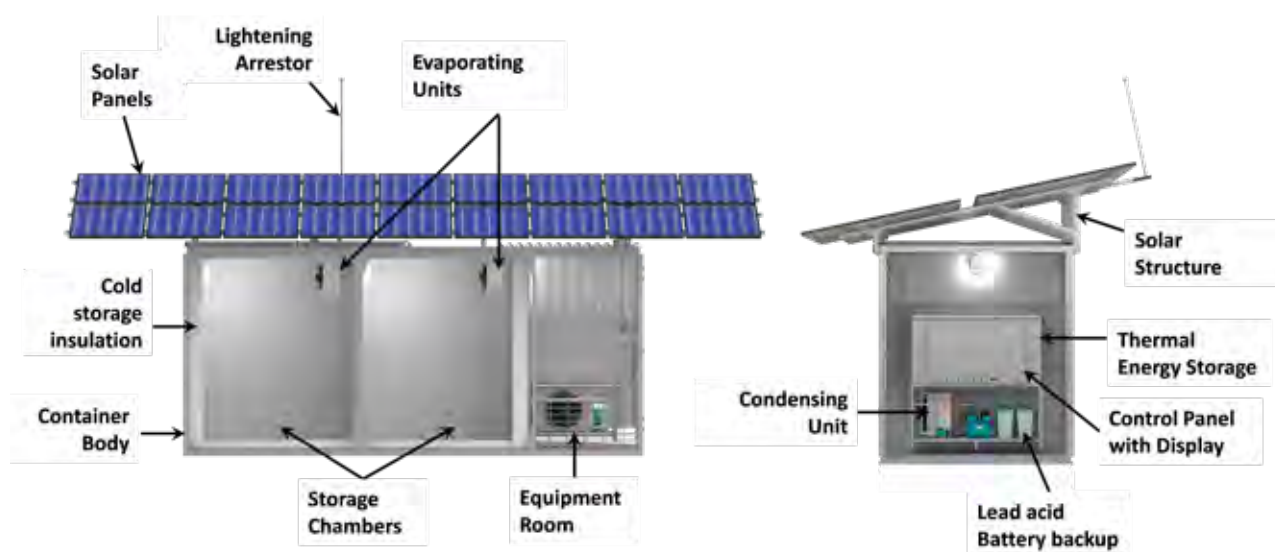
Figure 2: Typical layout for a multi-chamber solar cold storage
