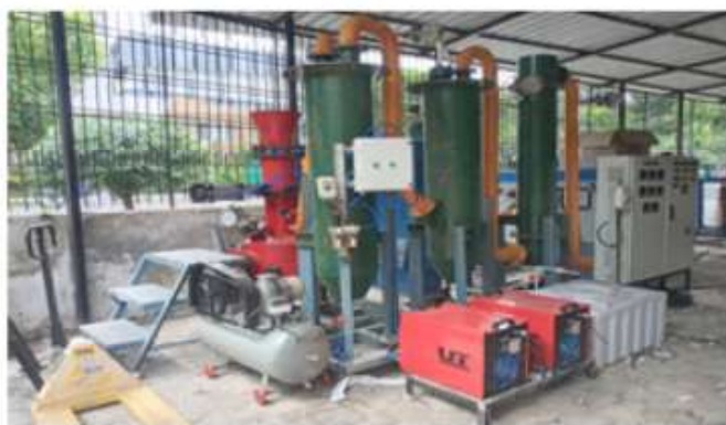
Fig. 7.6: Plasma reactor unit for biomass gasification being installed by IIT-Roorkee
