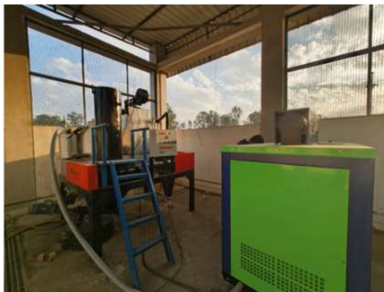
Fig.7.5: Agro-residue based downdraft gasifier with 10 KVA gen set
