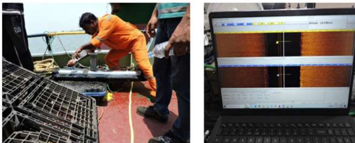
Fig. 9.8: Deployment of Side scan sonar and Data interpretation
