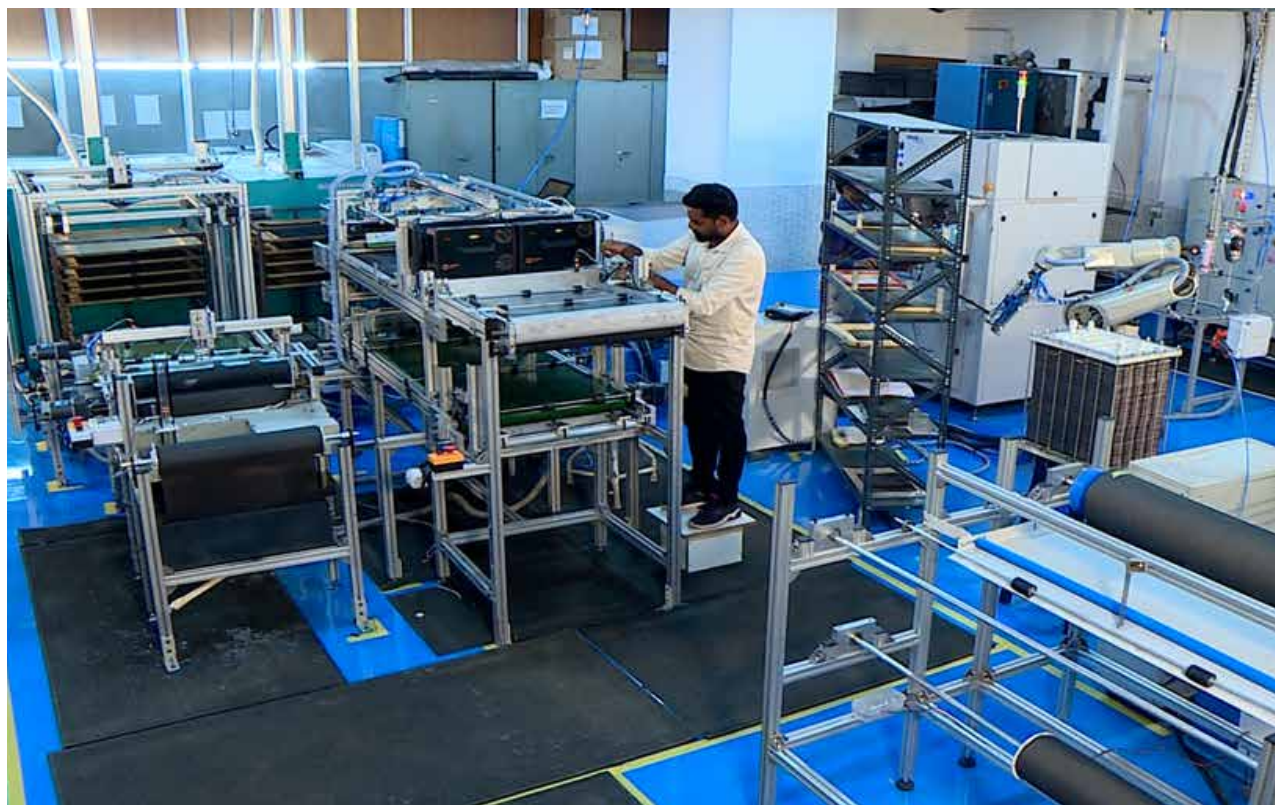
Figure 3. Established PEMFC components/stack assembly pilot line at ARCI-CFCT, Chennai
