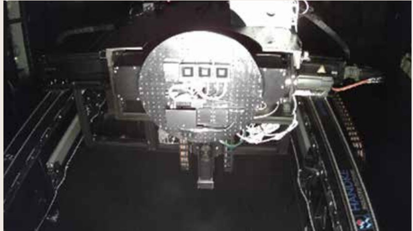
Figure 2. WPVS reference solar cells 009-2019 and 010-2019 used to assess the performance of the system
