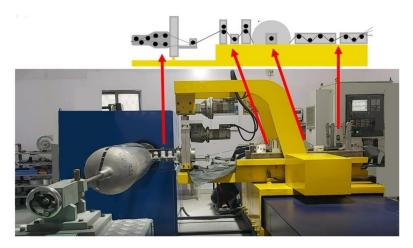
Figure 4: Filament winding machine
