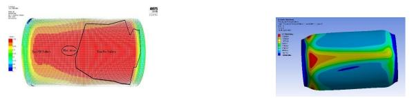
Figure 5: FEM Simulation results of Type III composite Cylinder
