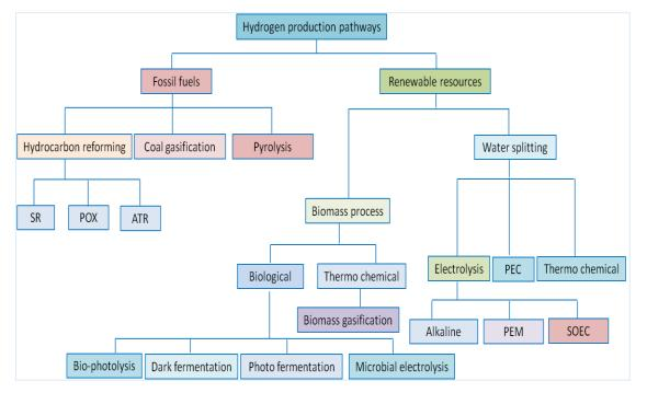
Figure 1: Various pathways for hydrogen production
