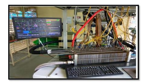
Figure 11: Testing of CSIR-3 kWe Fuel Cell Stack at Industry site (CSIR-NMITLI Program)
