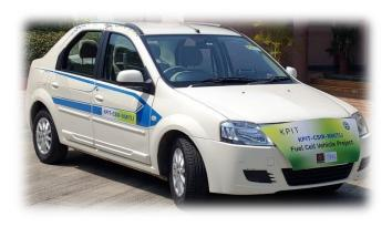
Figure 12: Testing of CSIR-10 kWe Fuel Cell Stack for Vehicular platform in collaboration with Industry(CSIR-NMITLI Program)
