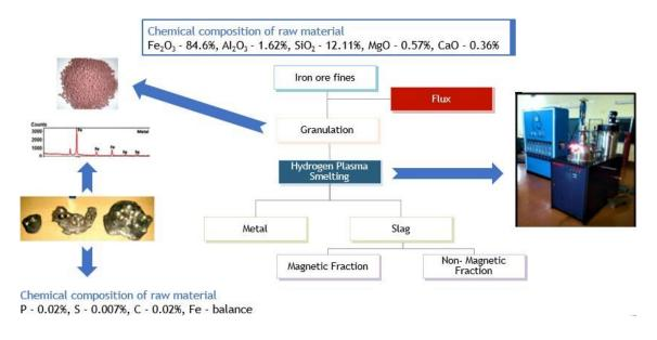
Figure 15: Process flow chart for green steel production
