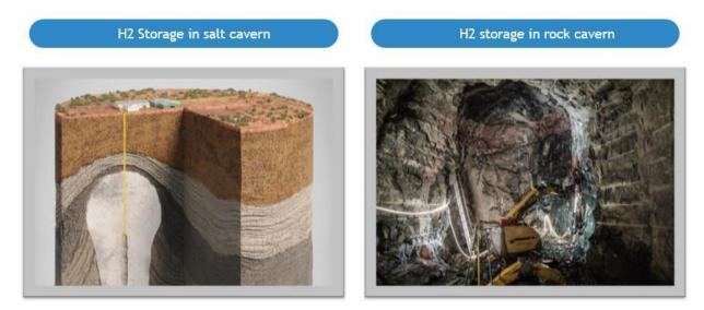
Figure 3:a). H<sub>2</sub> Storage in a salt cavern, b). H<sub>2</sub> storage in rock cavern (Source: Google)
