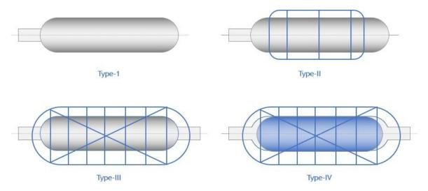
Figure 17: Different Types of Cylinders
