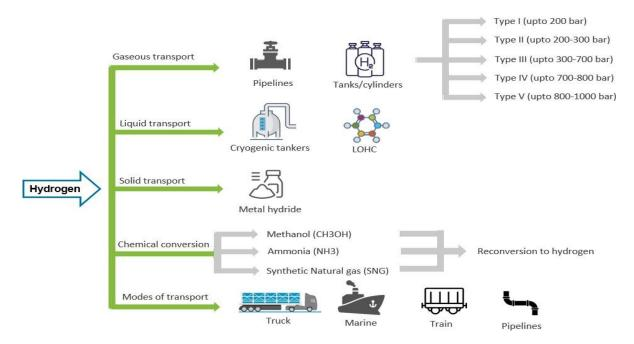
Figure 8: Pathways for hydrogen transport
