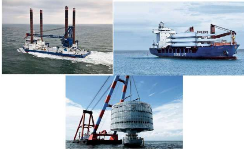
Figure 6-3: Types of specialized vessels such as: Installation (Jack up), multipurpose cargo, heavy lift. (Ref. 9)
