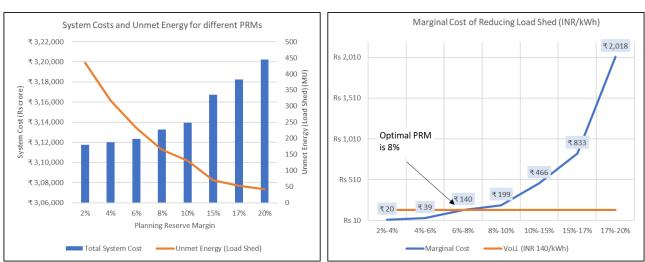
Figure 2: Illustration of Calculation of Marginal Cost of Reducing Load Shed
