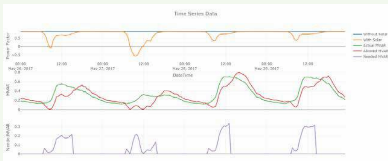
Figure 47: Solar Injection at Unity Power Factor (Source: CES analysis)
