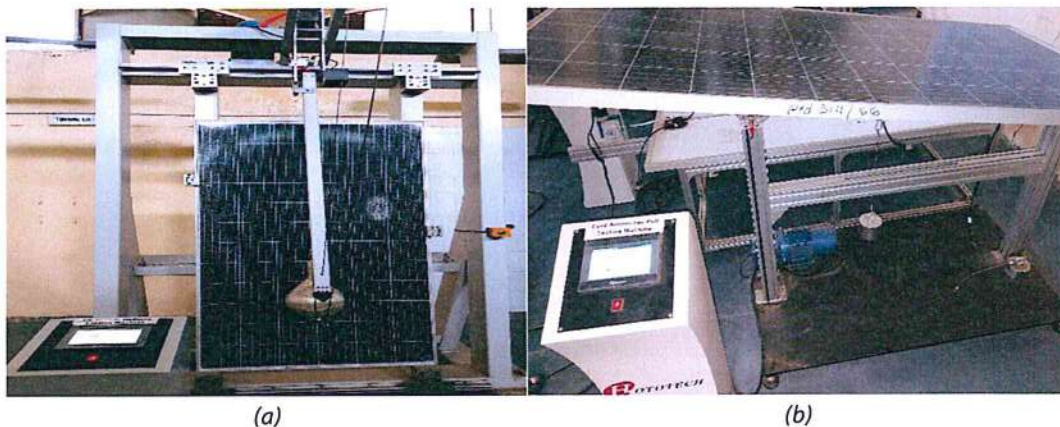
Fig. 10.2: Test equipment at Module Testing Lab (a) Module breakage tester and (b) Chord anchorage tester.
