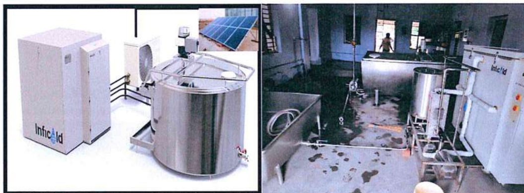
Fig. 10.7: Bulk Milk Chiller System
