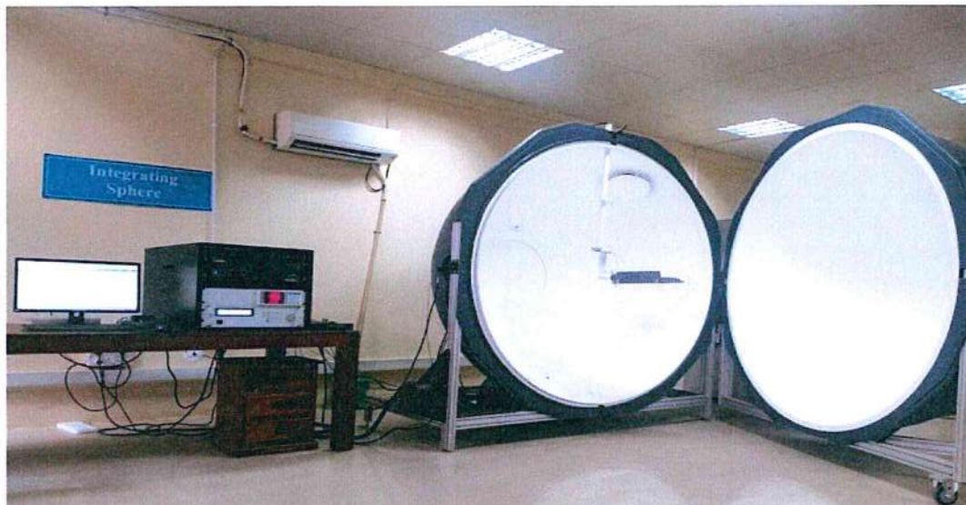
Fig. 10.3: Testing of Solar Street Lights with Integrating sphere system.
