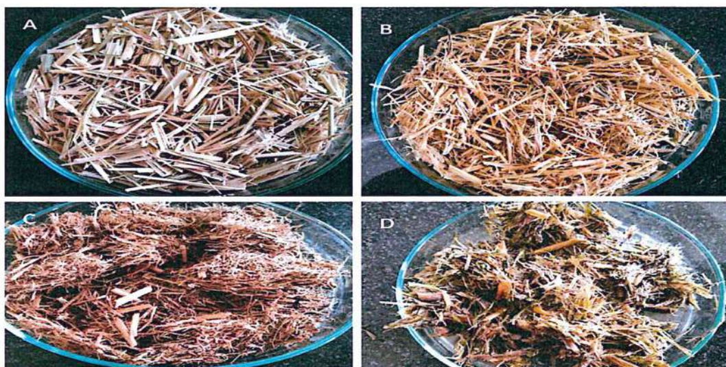
Fig. 10.18 A) Raw Kans Grass Biomass B) NaOH Pre-treatment C) Acid Pre-treatment D) Ammonia Pre-treatment
