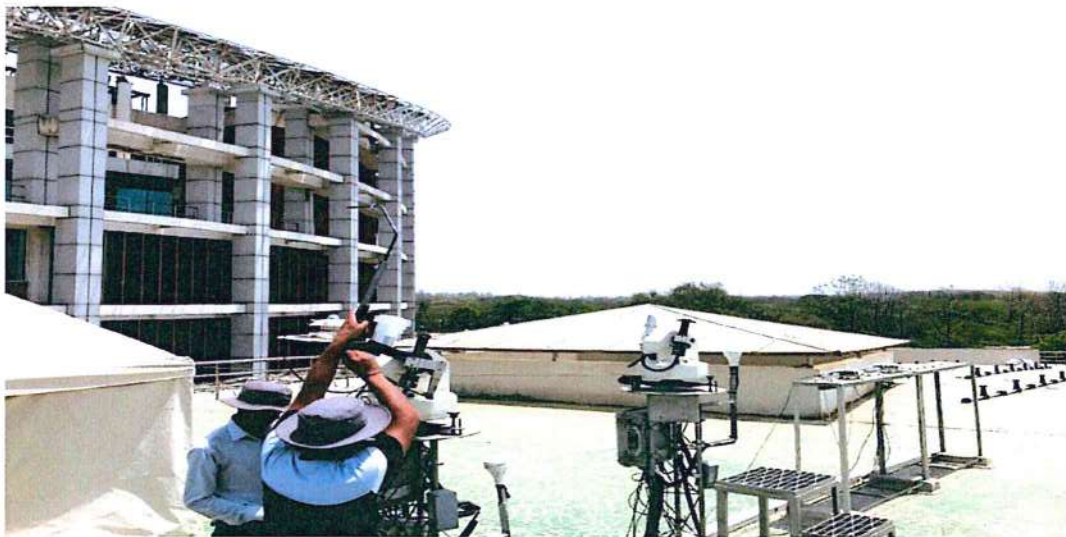
Fig. 10.11. Calibration of Radiometers at NISE (Project funded by MNRE)
