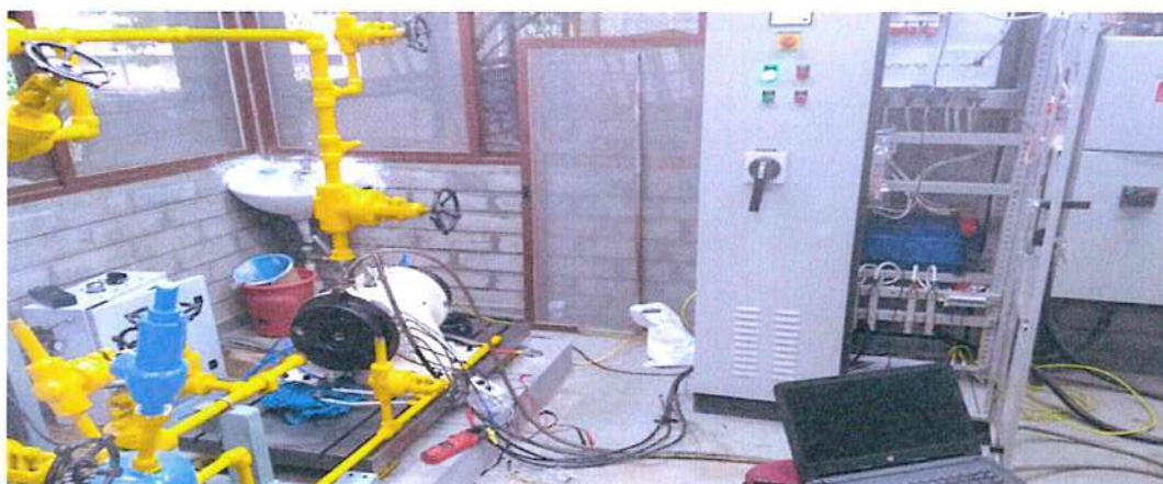
Fig. 7.12: Motor mode testing of the turbine-compressor assembly with generator
