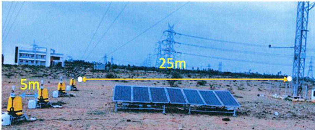
Fig. 7.16: LiDAR validation set up at WTRS, Kayathar, Tamil Nadu
