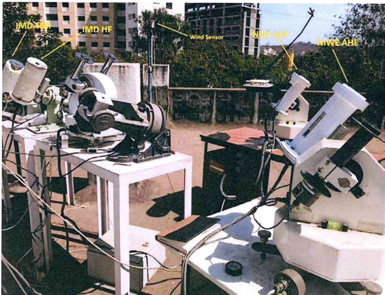
Round robin testing of Primary Standard Reference sensor from Calibration laboratory at NISE, NIWE & IMD Pune March 2018
