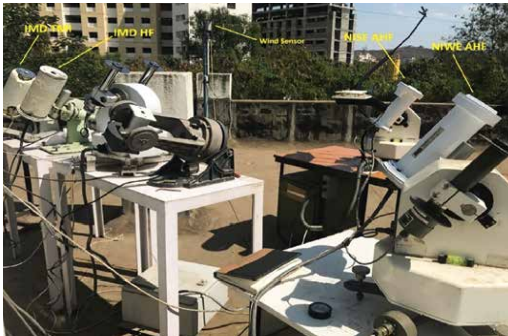
Round robin testing of Primary Standard Reference sensor from Calibration laboratory at NISE, NIWE & IMD Pune March 2018.
