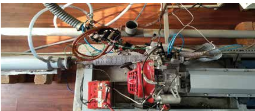
Commercial SI engine setup (Honda GX 200) –turned into biogas fueled SI engine at IIT Guwahati
