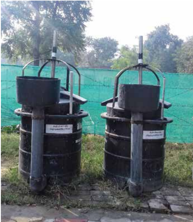
Biogas production on hydrothermally pre-treated paddy straw in 300 L daily feed anaerobic digesters at IIT, Delhi
