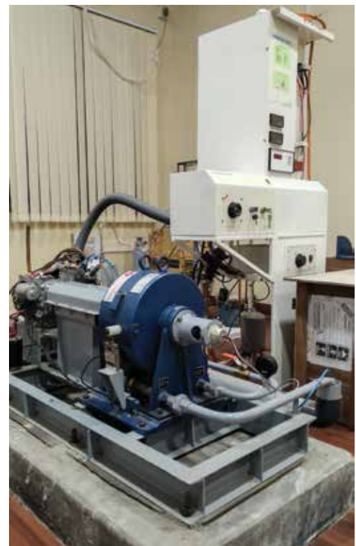
Commercial SI engine setup (Honda GX 200) –turned into biogas fueled SI engine at IIT Guwahati
