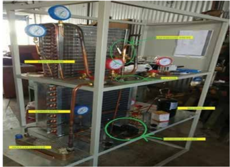
Experimental set up of desiccant and ejector based environmental friendly Air conditioning system at Maharashtra Institute of Technology, Pune
