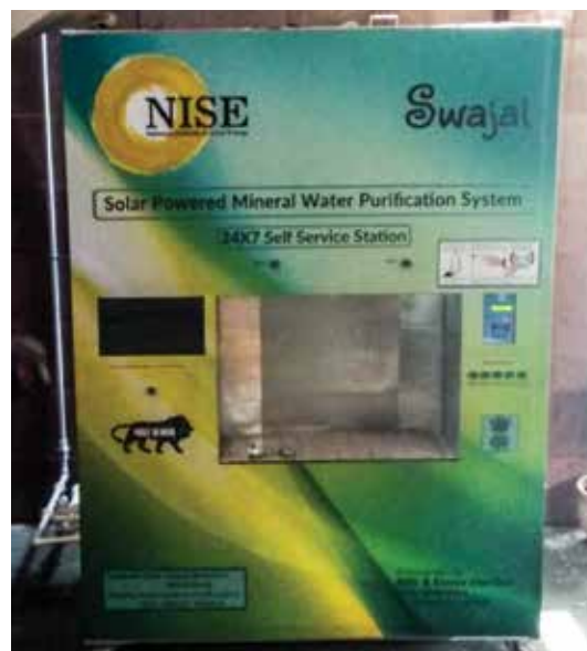
Fig. 5a second prototype (fully DC, low power consumption, 100 LPH) at Aditya Bhavan, NISE
