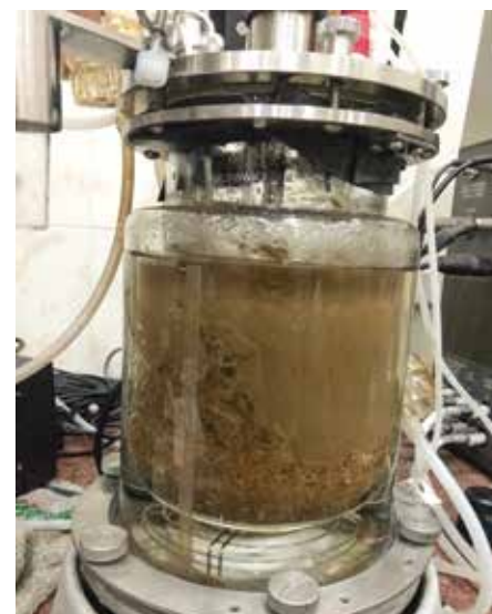
Ethanol production from ammonia pre-treated bagasse in SSF
