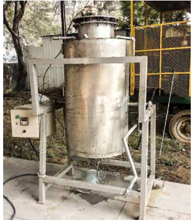
50 L capacity field scale hydrothermal reactor at IIT, Delhi
