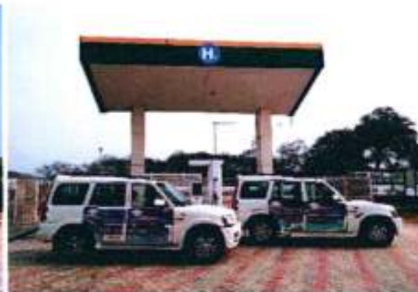
H 2 -Diesel Dual Fuel Vehicles developed by M&M
