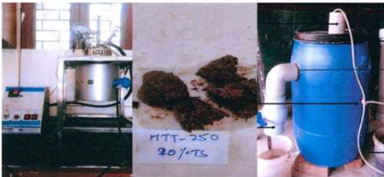
Laboratory scale hydrothermal reactor at IIT, Delhi
