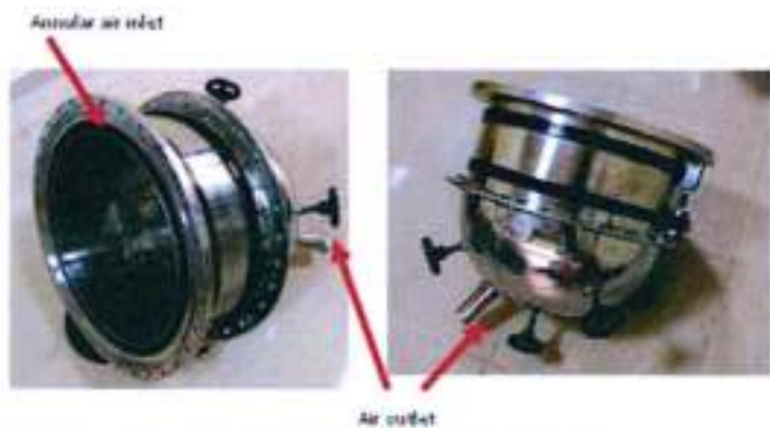
Solar receiver fabricated at IISc, Bangalore
