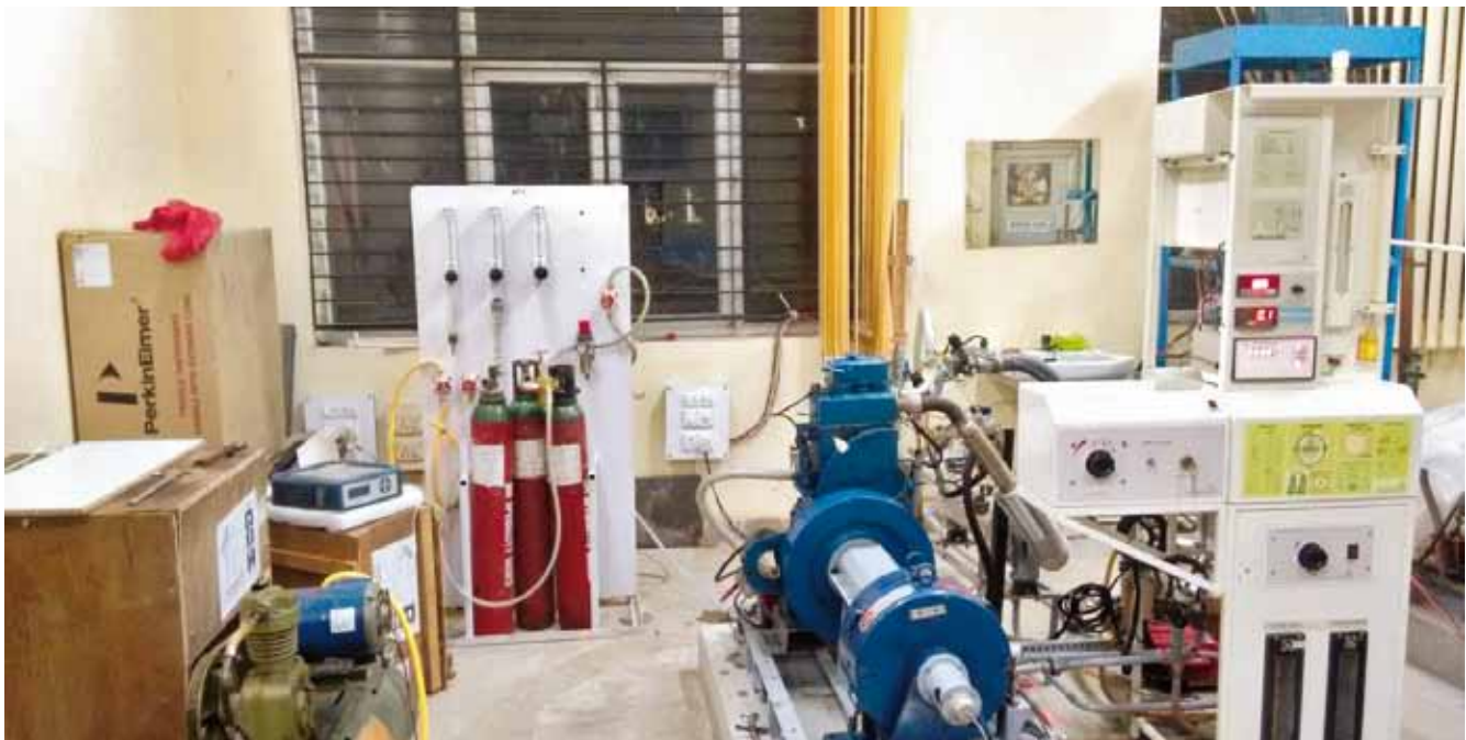
Experimental Set-up for Biogas and Methane Testing at IIT, Guwahati Laboratory
