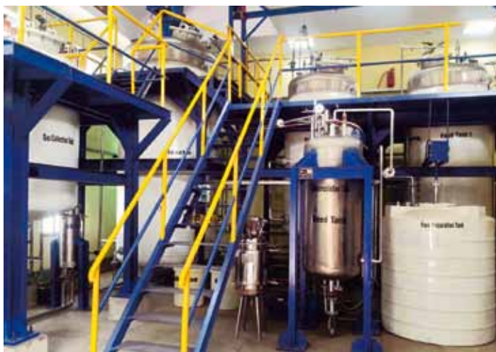
10 cu.m Pilot plant for biohydrogen production at IIT Kharagpur
