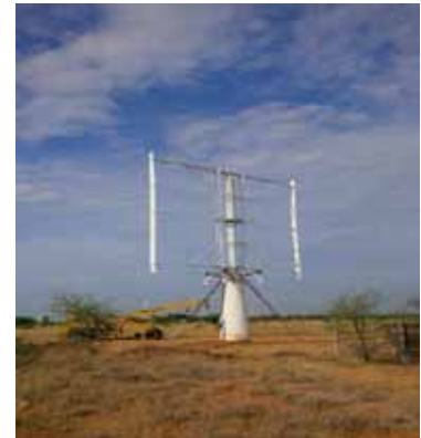
Testing of 15 kW small vertical axis wind turbine
