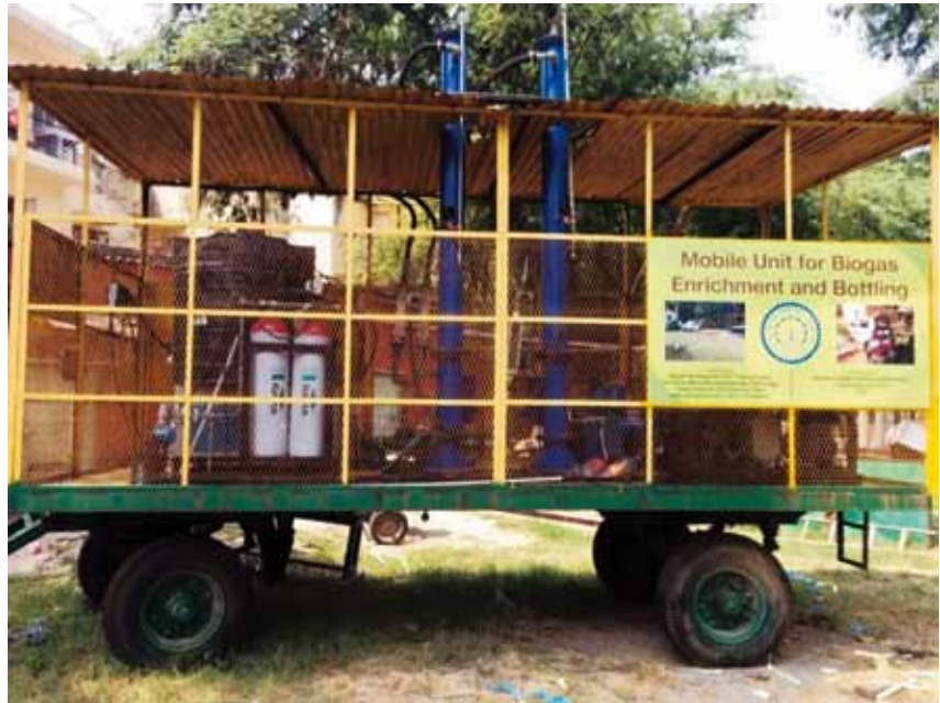
Biogas purification and bottling unit at IIT Delhi
