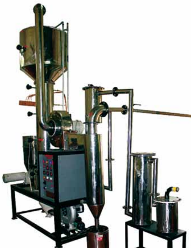
Fluidised Bed Biomass Gasifier developed at NIT Calicut
