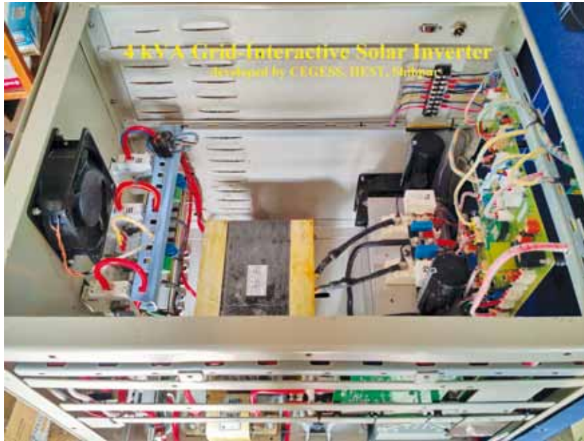
A 4kVA Grid-Interactive Solar Inverter developed by CEGESS, IEST, Shibpur, Kolkata
