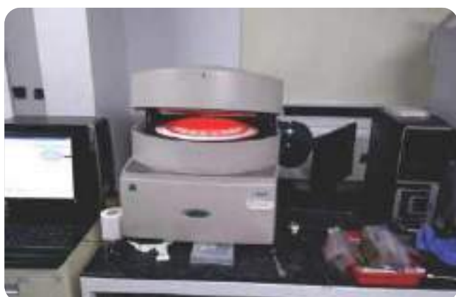
Figure 201: Apparatus used for testing crop samples for GCV
