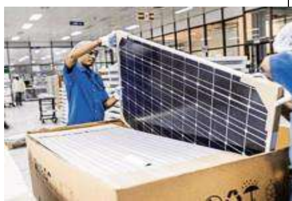
Figure 27 Solar module handling and stacking
