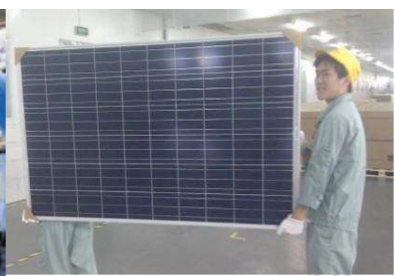
Figure 28 Solar PV Module handling
