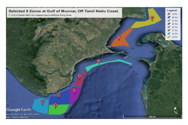
Fig. 1: Demarcated Offshore Wind Energy Zones at Tamil Nadu
