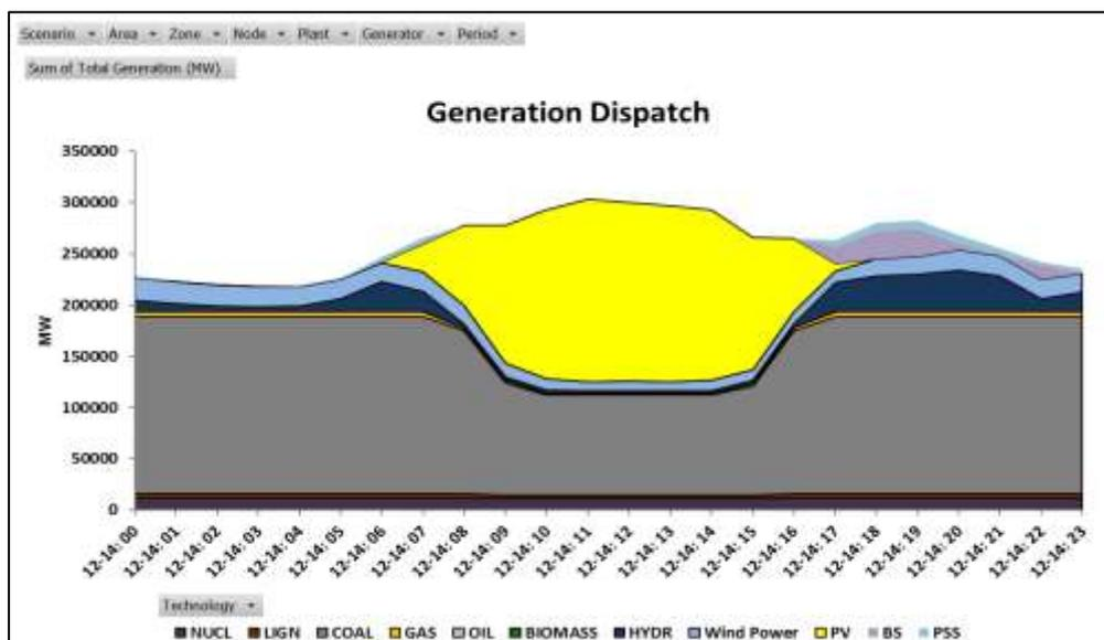
It has been observed that during this critical day when energy demand of the system is minimum, the demand is likely to be fully met with the supply side options as per the long-term studies. It is observed that despite hydro and wind generation being relatively less, RE absorption on this day is likely to be around 97.19%. RE generation dispatch and absorption on this day is shown in the **Exhibit 20**.
