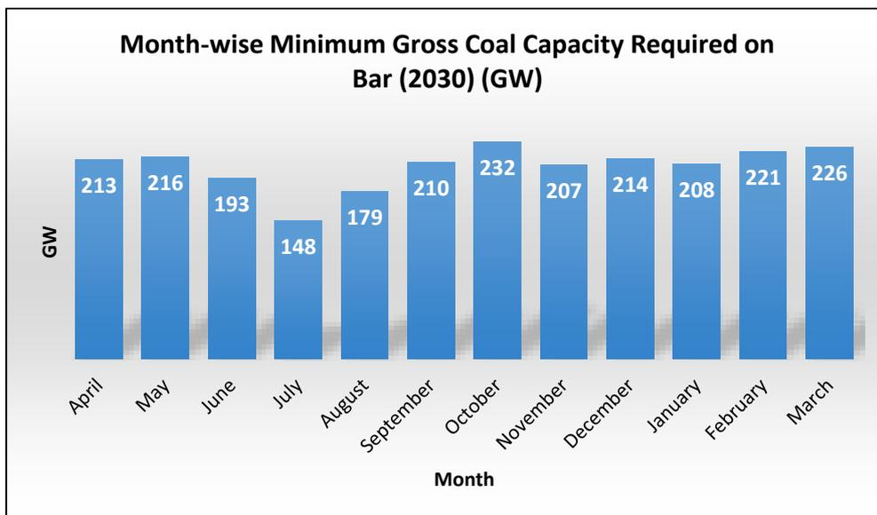
It can be seen from the **Exhibit 32** that more than 160GW of coal based capacity is required to be on bar for more than 50% of the time for the whole year.
