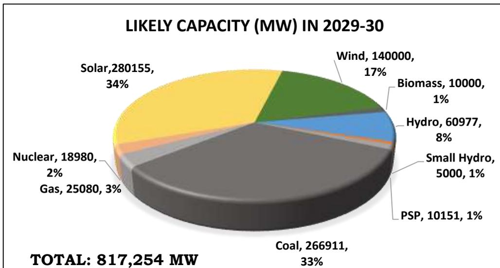
The projected gross electricity generation (BU) during the year 2029-30 is likely to be 2,518 BU comprising of 1,393 BU from Thermal (Coal, Gas and Lignite), 801 BU from RE Sources, 207 BU from Hydro, 4.4 BU from PSS and 113 BU from Nuclear as shown in **Exhibit 9**.
