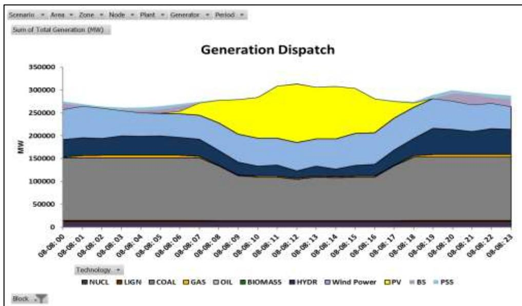
It has been observed that the day when solar generation is minimum, the demand is likely to be fully met with the generation capacity mix obtained from the long term studies. This is due to significant availability of hydro and wind energy during monsoon season. It has been observed that RE generation is fully absorbed on this day as shown in the **Exhibit 18**.
