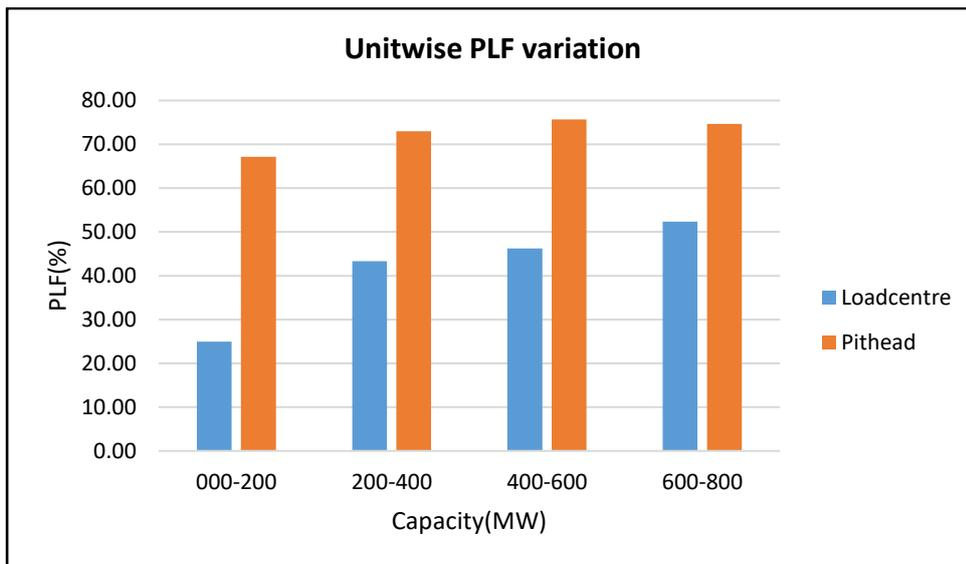
From the graph, it can be concluded that the load centre small size units may be required to run at low PLF of about 20% . Small sized units may be required to undergo flexible operation frequently compared to pit head large sized units.
