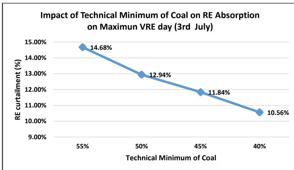
During the course of above analysis, it was observed that RE absorption can be increased with reduction in minimum technical load, thus increasing flexible operation of thermal power plants. However, this entails investment for technological upgradation in coal based power plants. An increase of approximately 1.5 % in the RE absorption was observed for every step of 5
