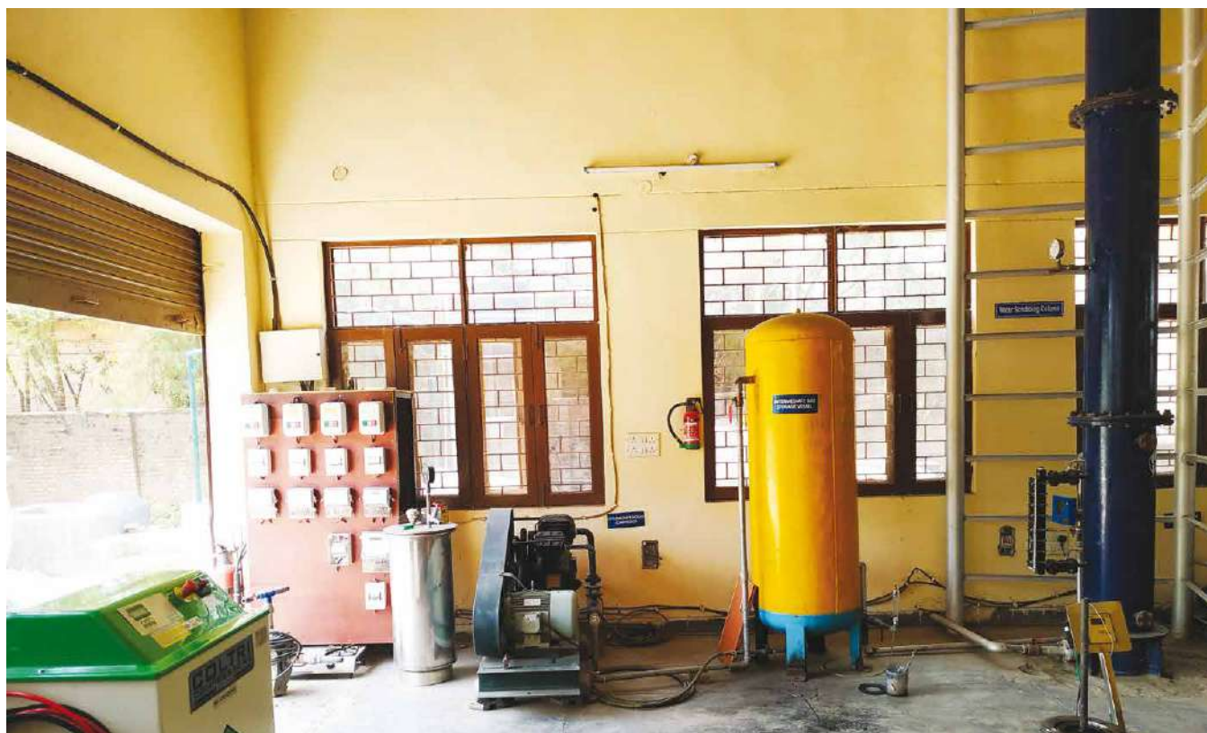
» Water scrubbing technology for biogas upgradation plant installed in Biogas Enrichment and Bottling Lab, CRDT, IIT Delhi
