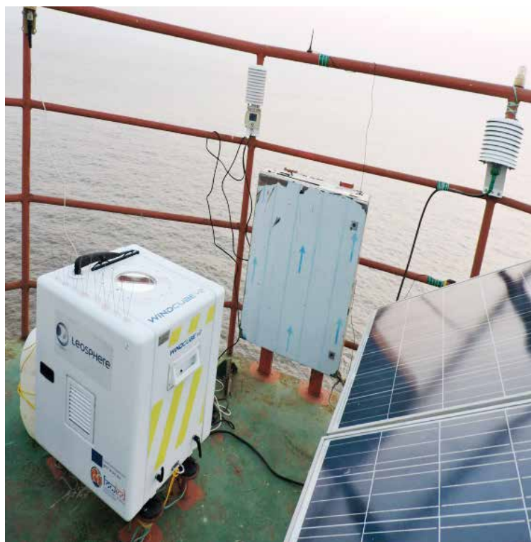
» Offshore LiDAR structure and LiDAR off Gujarat coast (23 km from Pipavav)
