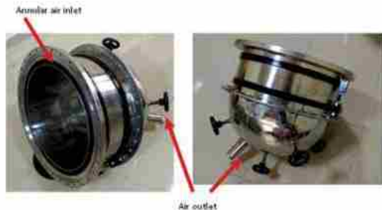
Solar receiver fabricated at IISc, Bangalore
