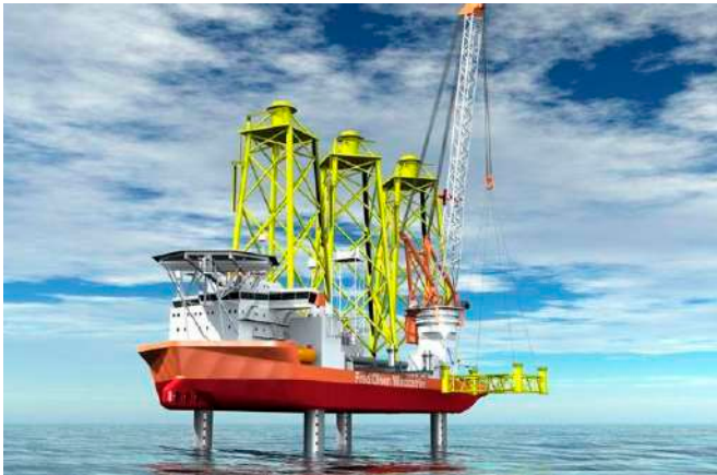
Figure 59 - Large DP2 WTIV - Fred Olsen Windcarrier's Bold/Brave Tern pre-piling jackets
