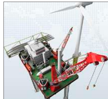
Figure 58 - A small DP2 WTIV Seajack's Kraken
