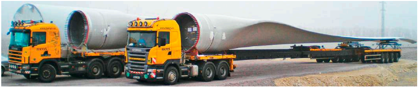
Figure 26 - Blade handling trailers for road haulage and handling in port estates
