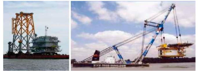
Figure 81 - Barge for transport and SHLV for installation of OSS foundation and topside
