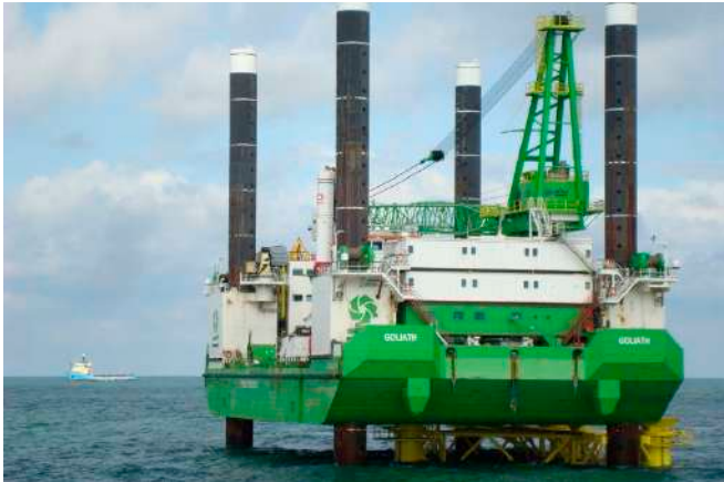
Figure 72 - Small pile-driving jack-up, with yellow under-slung pre-piling template
