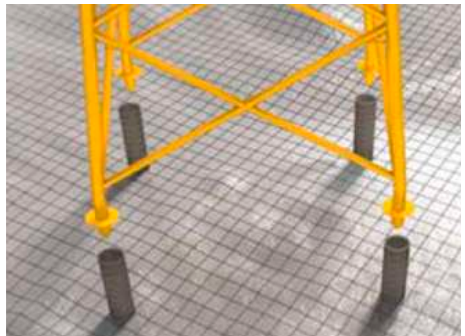
Figure 73 - Jacket leg stab-ins at point of insertion into pre-piled foundation
