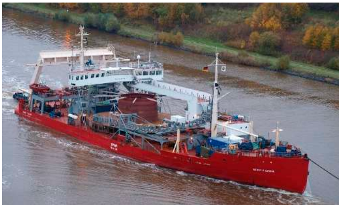
Figure 82 - Dedicated cable laying vessel for export cable installation
