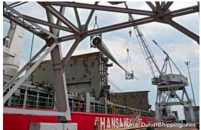
Figure 29 - Port crane blade load out
