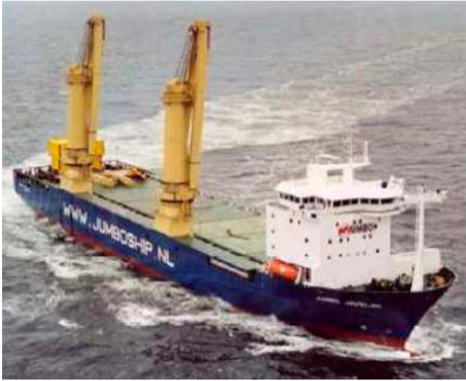
Figure 79 - Heavy lift cargo vessel, used for wtg transportation
