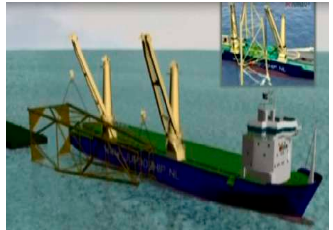
Figure 63 - Heavy lift cargo vessel - jacket installation
