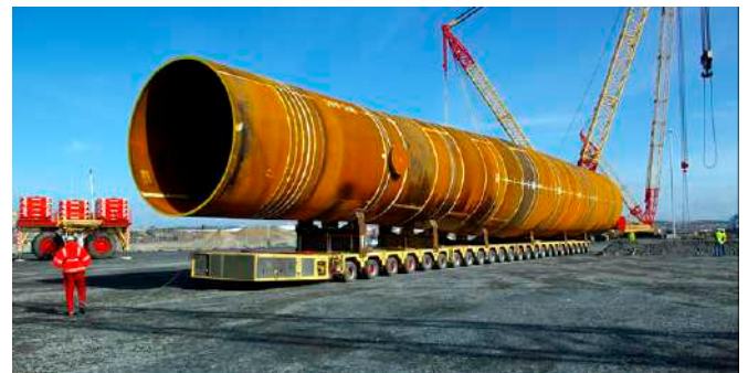
Figure 41 - Monopile onshore transport using SPMTs
