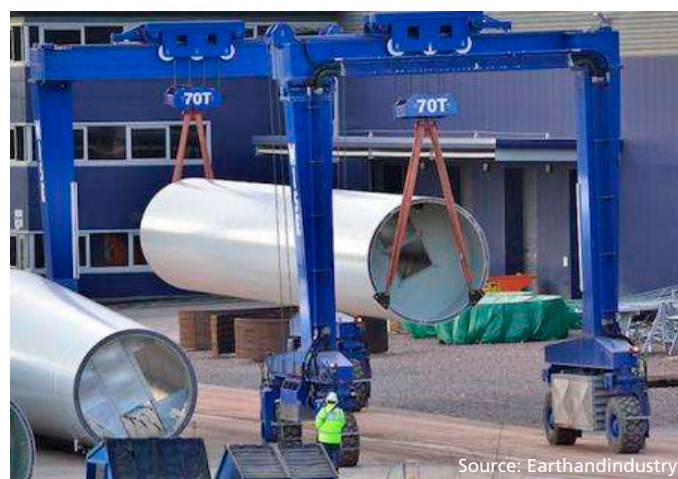
Figure 33 - Tower section transportation
