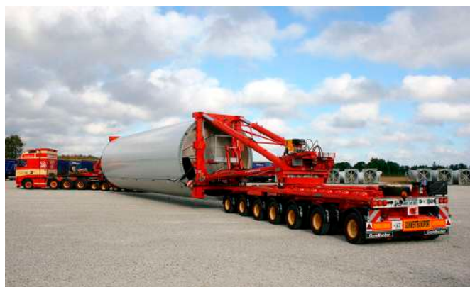
Figure 32 - Goldhofer RA3 tower haulage unit
