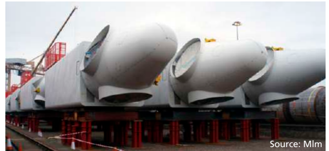
Figure 95 - Nacelle storage at port
