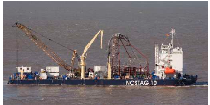
Figure 85 - Cable transportation and installation
