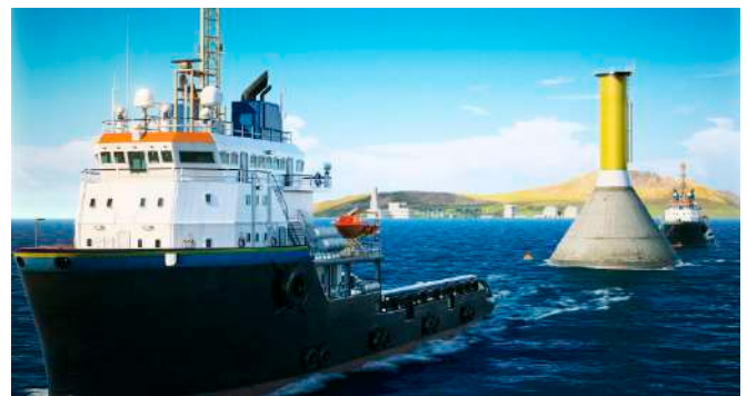
Figure 78 - Towing a floating Gravitass GBS foundation
