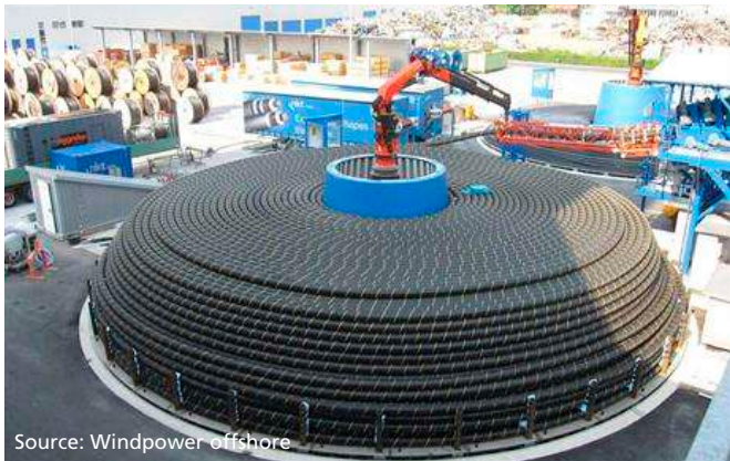
Source: Windpower offshore Figure 50 - Offshore wind cables stored onshore
