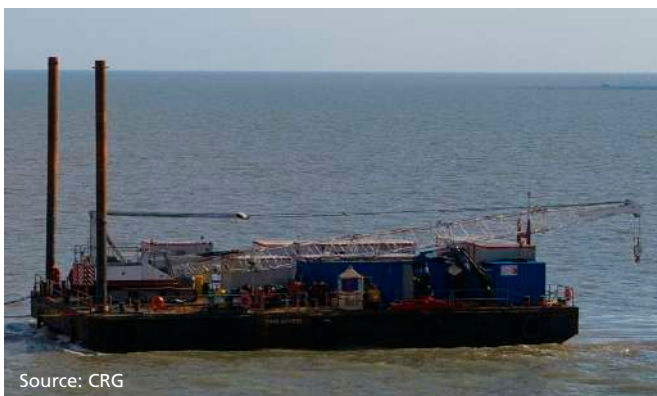
Figure 54 - Dumb barge with spud-legs, and crawler crane
