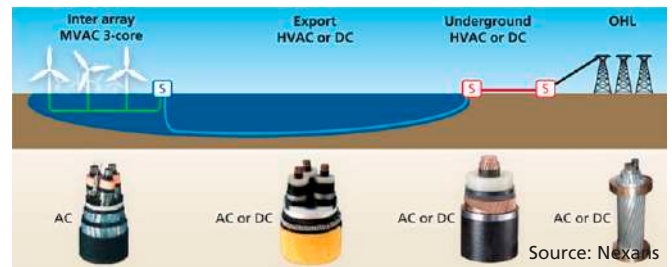
Figure 13 - Offshore wind export and array cable types
