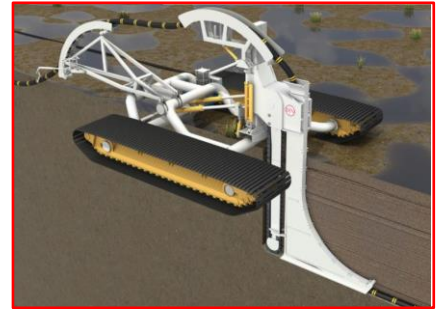
Figure 37 Example of post burial method
