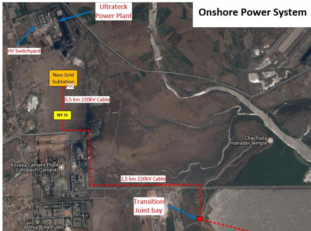
Figure 93 Option 2 – Onshore Cable Route & Substations Suggested
