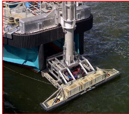
Figure 42 Mobilisation of sonar at survey vessel
