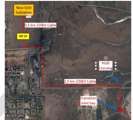
Figure 101 Option 2 – 220kV onshore cable route
