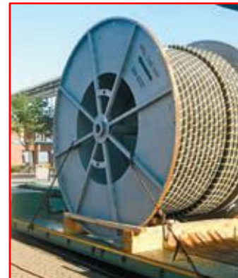
Figure 16 Transport rigging of array short length on cable drum
